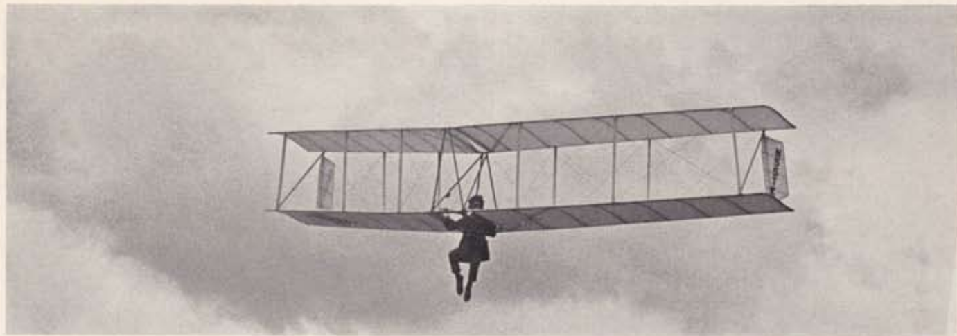
(This page) Taras Kiceniuk, a 17-year old from Los Angeles, and his Icarus II tail-less biplane, which holds the hang-gliding endurance record of over an hour. It is built of aluminium tubing with styrofoam ribs. Control is by tip-mounted rudders.
