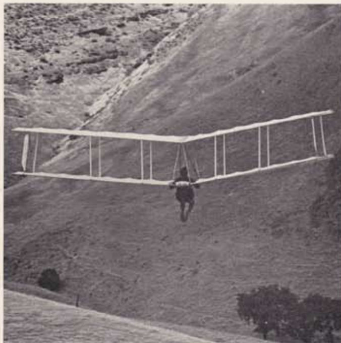
(This page) Taras Kiceniuk, a 17-year old from Los Angeles, and his Icarus II tail-less biplane, which holds the hang-gliding endurance record of over an hour. It is built of aluminium tubing with styrofoam ribs. Control is by tip-mounted rudders.
