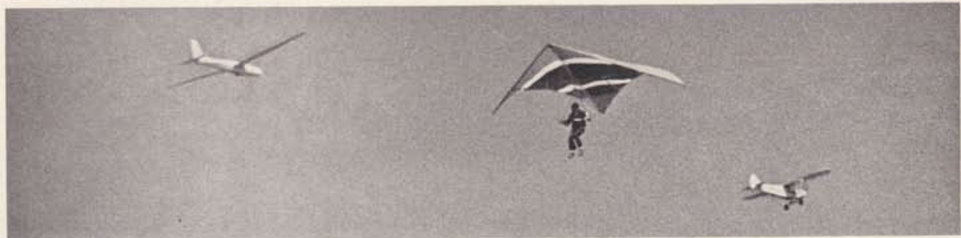
(Top) Launching a Rogallo that features leading-edge slots for (hopefully) better low-speed manoeuvrability.
