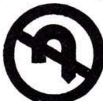
BOTTOM LANDING PROHIBITED
