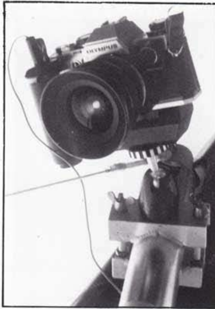
Camera mounted on the cross boom of Tony Hague's Silhouette. Olympus OM10, winder, 18mm. Sigma lens.
