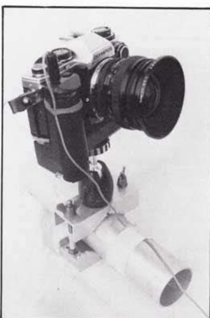
Glider mounted camera assembly posing on a piece of tubing. Olympus OM10, winder, 18mm. Sigma lens.
