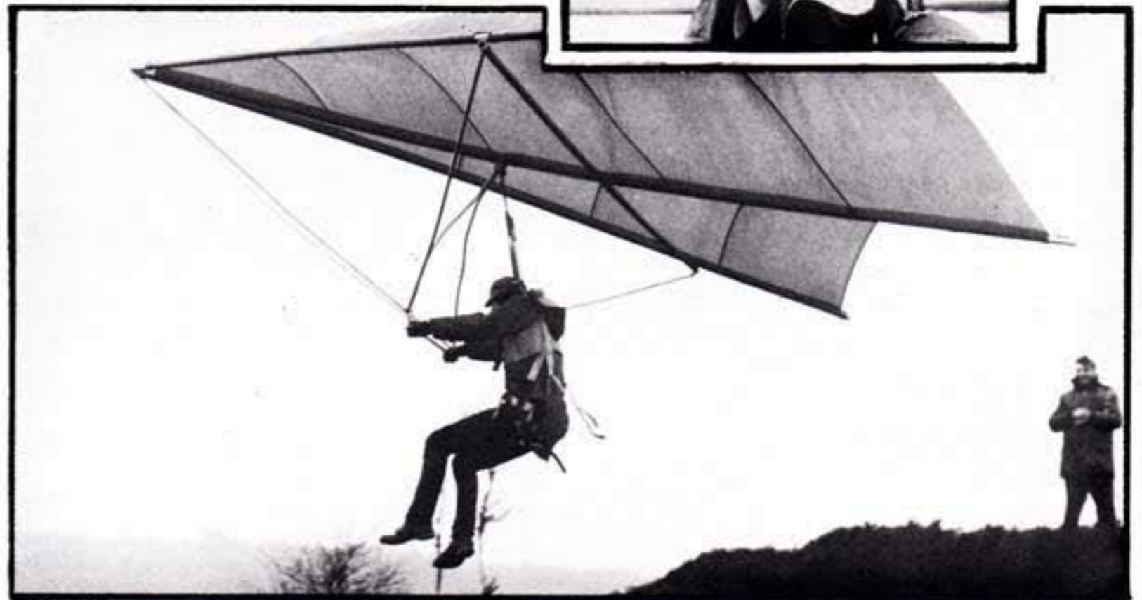
Top — Mr. Regan himself. Below — it actually flies. Note the very bent uprights!
