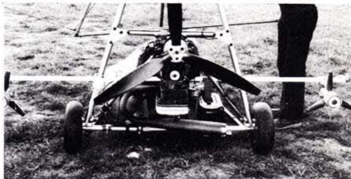
Picture shows the Buckle-May spray gear fitted to a trike
