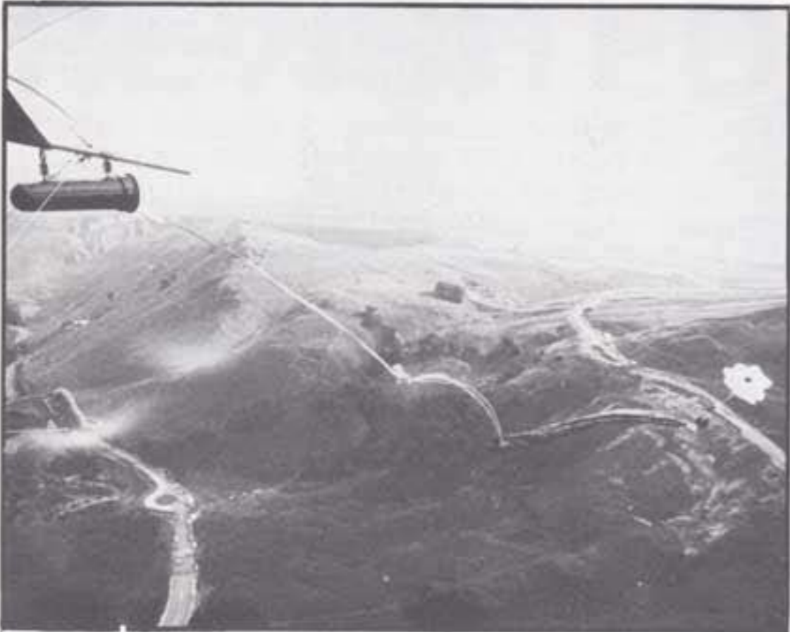
3: 2.6 seconds - system now fully streamed with bridle just beginning to lift clear of the sail.
