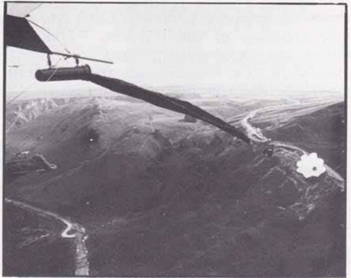
2: 1.6 seconds - drogue now pulling main canopy clear of container.
