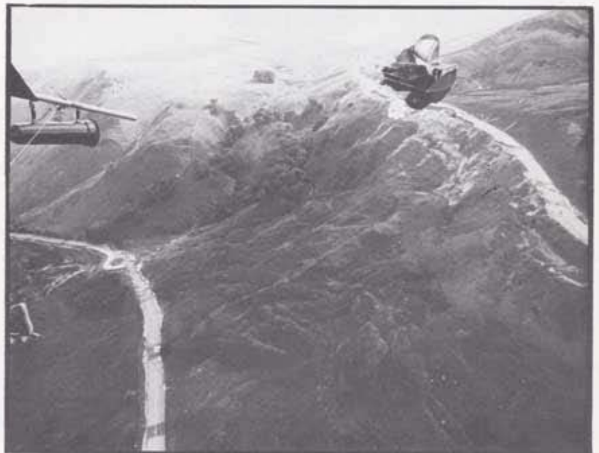
4: 4 seconds - bridle tensioned: canopy beginning to inflate.
