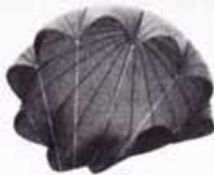
Bottom right — Drogue chute collapses as main canopy robs it of air. Special design of main canopy evident from conical shape.
