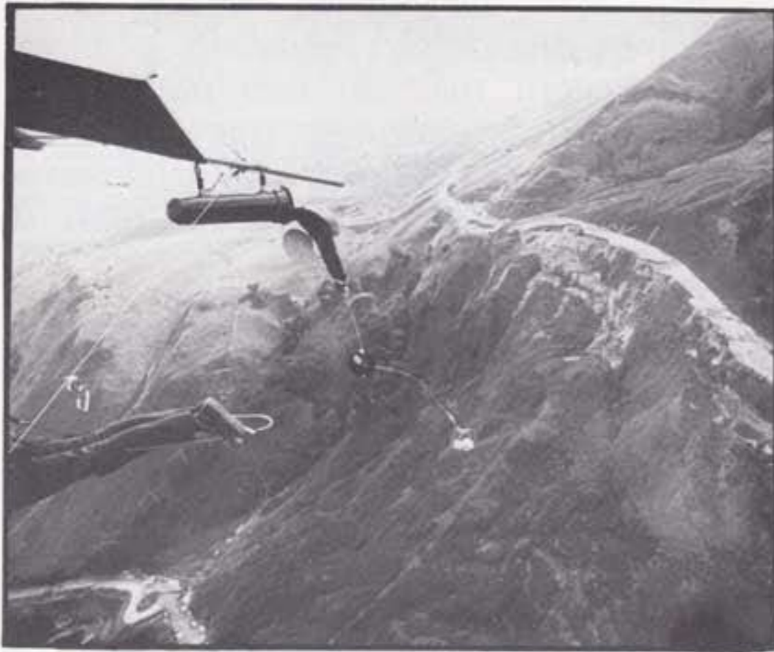
1: 0.2 seconds - the spring unit (circular object between pilot chute and main canopy) has flipped off the end cover and fired the drogue into the airstream. The main canopy is already starting to emerge even though the drogue has yet to inflate.
